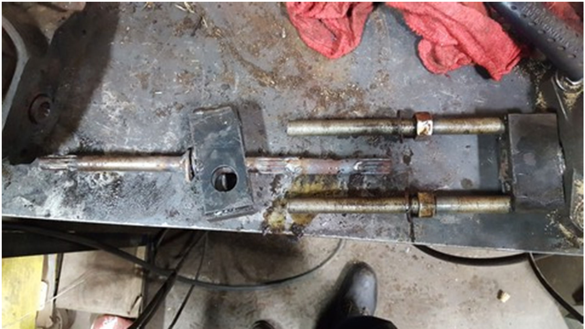
The shaft after being pushed out of the pinion.
