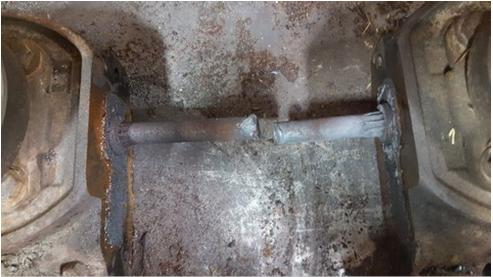
The two modules with the drive shaft cut and the spacer removed
